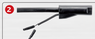
2 Left and right rear lamp plug integrating twin core marker cable with plug connectors.
